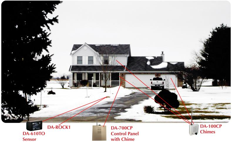
This home owner did not want to trench cable, nor did she want to run wiring for hard-wired chimes in the house. In addition to the chime alert, she wanted to trigger flood lights, for a specific time, when vehicles were detected. Finally, she wanted to add another sensor at a workshop on the property and differentiate alerts with different chimes for the driveway and the shop. Mier's Tech Support Team helped her choose the following:
