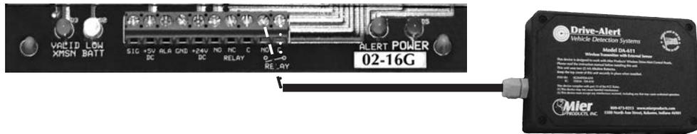
**To install the DA-REPEATER** to a **DA-500**, attach one wire to the "NO" terminal and the other to the "C" terminal as shown here:
