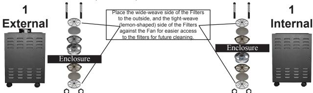
Once you have chosen to mount your fan internally, or externally, please follow these steps in assembling your fan and mounting it onto the enclosure.
